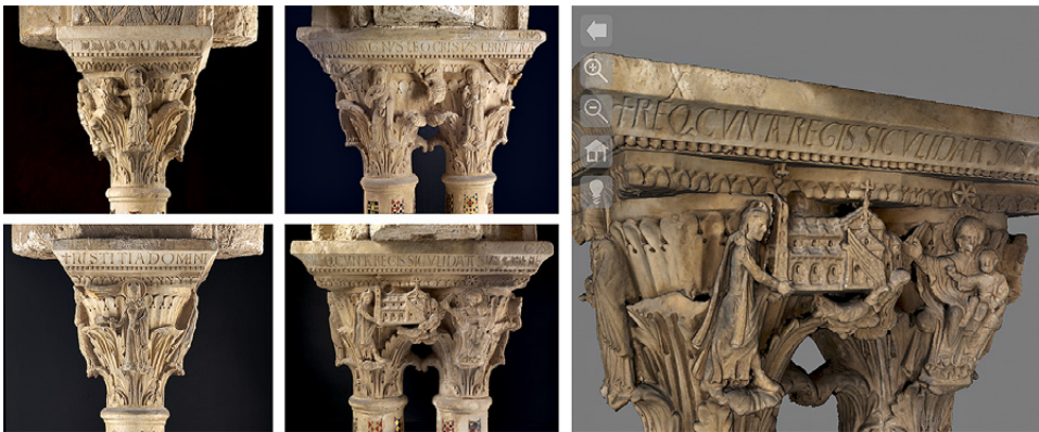
Fig. 2 – An example of the Monreale cloister, west side, capital no. 8; left: the set of photos acquired; right: the related 3D model, produced with active 3D scanning technology.
