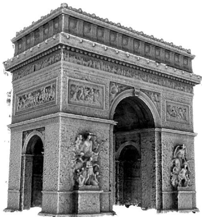
Fig. 6 – A 3D model reconstructed from just a sequence of approximately one hundred high resolution photos. The reconstruction was performed using the tools developed within the EU IST NoE “Epoch”.
