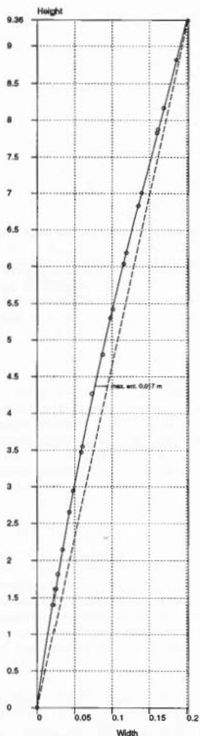
Fig. 1 - Parthenon: *entasis* of peristyle column. Third degree interpolation.
