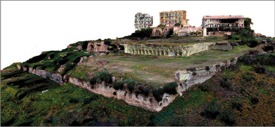
Fig. 2 – Post-processed point cloud without olive grove (elab. Authors).
