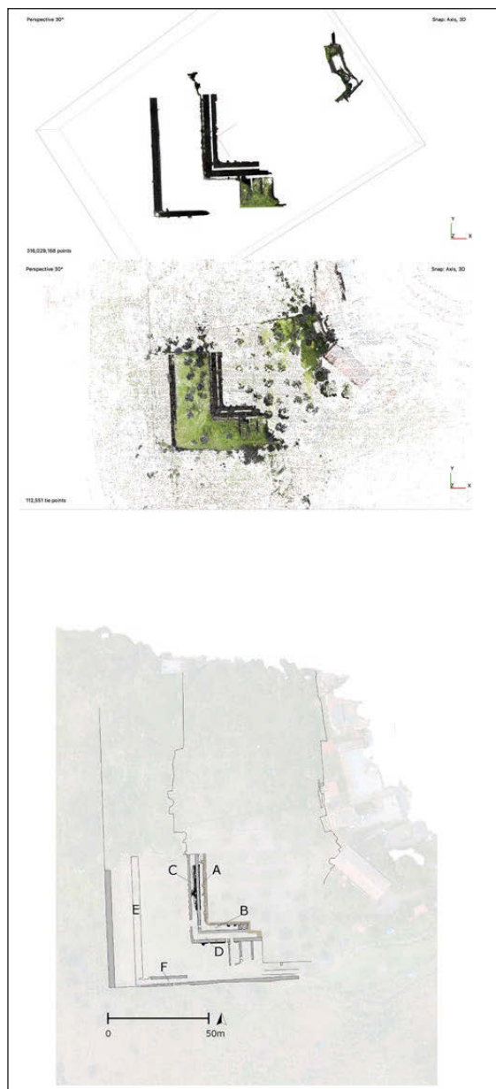
Fig. 8 – Integration of drone and laser scanner point clouds within the Brutus Villa Project: top, isolated substructiones ; bottom, substructiones integrated within the entire complex through drone survey plan of the ongoing work carried out during the first archaeological campaign of the Brutus Villa Project (elab. Authors).
