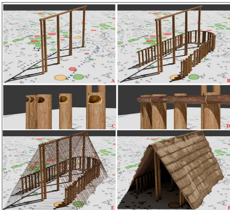
Fig. 5 – A) Placement of the central axial posts and ridge beams; B) perimeter posts and base posts; C-D) detail of the socket carved into the perimeter posts to receive the base posts; E) positioning of horizontal and vertical beams; F) roof covering made of bundled vegetal material.
