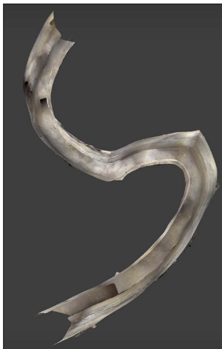
Fig. 6 – Augustan aqueduct at Bagnoli: top view of the junction between two digging teams, between adits R7 and R8 (Cocceius Association).
