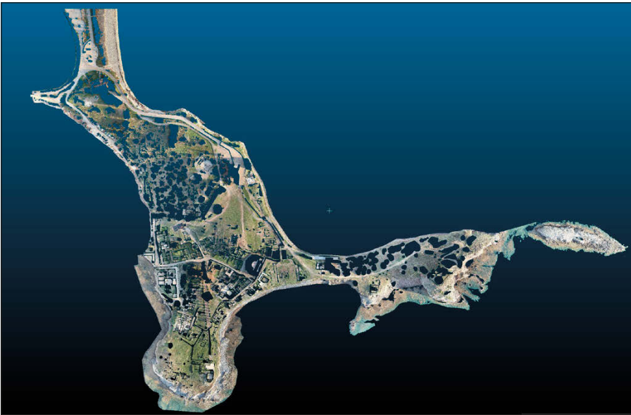
Fig. 3 – The cloud resulting from the non-ground point deleting activity; a considerable part of the cloud has been removed.
