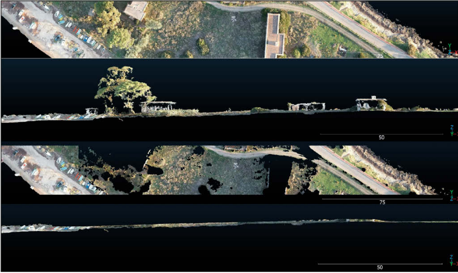
Fig. 2 – Processing workflow; from top to bottom: azimuthal view of the area; side view of the cloud before segmentation; azimuthal view of the point cloud after segmentation and side view of the cloud after segmentation.
