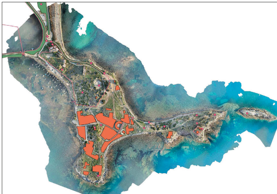
Fig. 6 – Orthophoto of the site with overlaid vector elements (excavation areas and Regional Trigonometric Vertices) of the Regional Technical Map (CTR) of Sardinia (reference system EPSG 3003).
