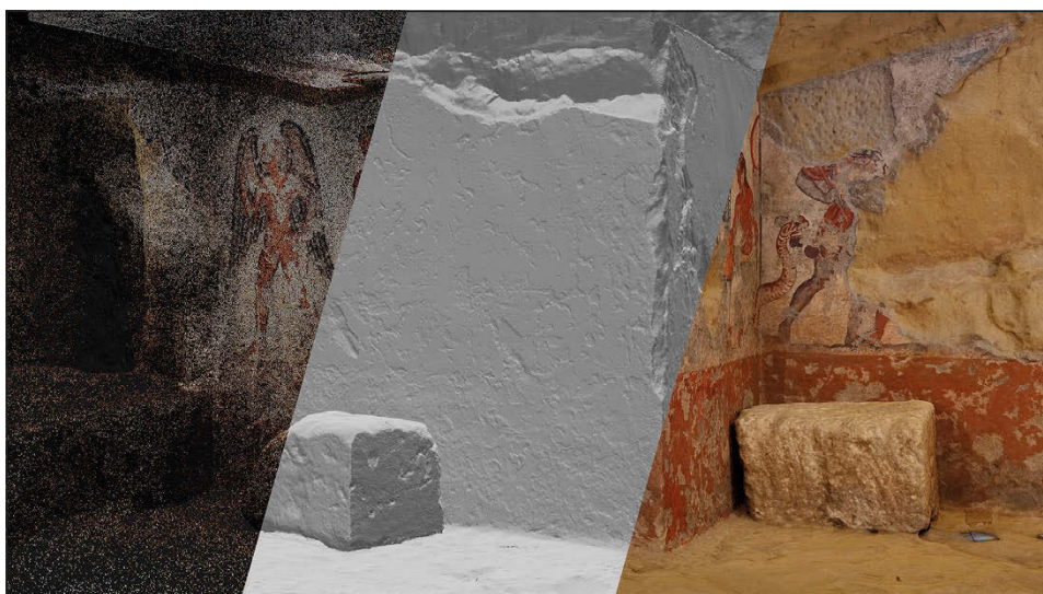
Fig. 9 – 3D digitization processes, from left to right – point cloud, shaded photogrammetric model, textures. Tomb of Orcus (Alban-Brice Pimpaud).
