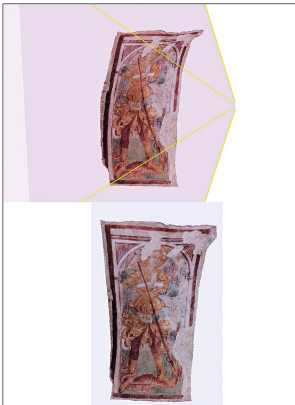
Fig. 4 – Texture mapping process of the main representation of the archangel Michael; more than 20 control points were used to accomplish the camera calibration.
