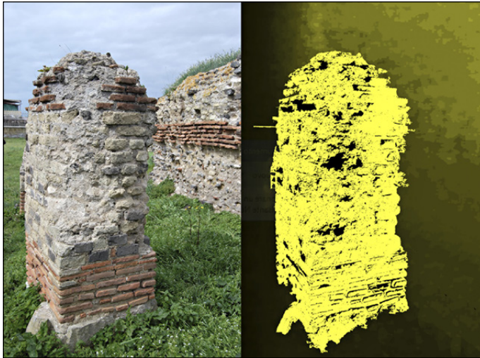
Fig. 3 – RGB-D scan survey: colorimetric information (right) and depth map (left).
