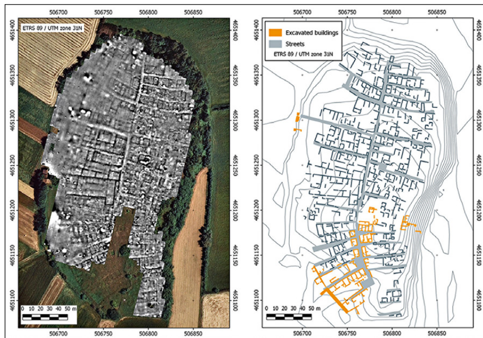
Fig. 2 – Gradiometer response map (Eastern Atlas) and interpretation diagram of the geophysical data from Illa d'en Reixac (after GARCIA-GARCIA, DE PRADO, PRINCIPAL 2016).
