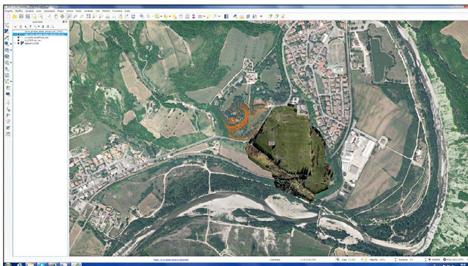
Fig. 2 – The three sources of elevation data: a) in green contour lines of the recent aerophotogrammetry, b) in orange acropolis contour lines and c) in dark green detailed photogrammetric survey by drone.
