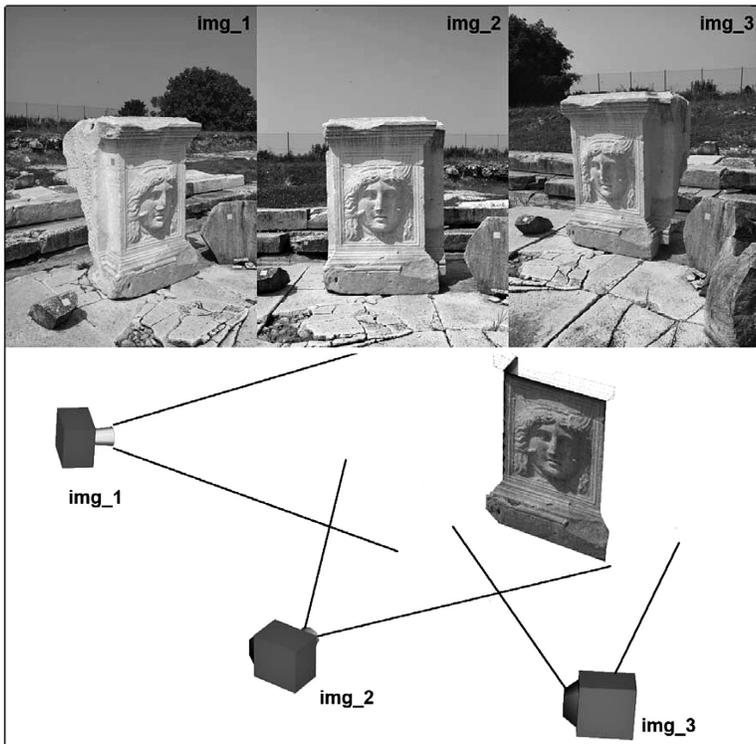
Fig. 3 – Example of the three photographs of the object and virtual representation of the original position of the camera for each photo.
