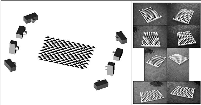
Fig. 1 – Design showing position and orientation of cameras during the photography of the calibration panel, and example of images.
