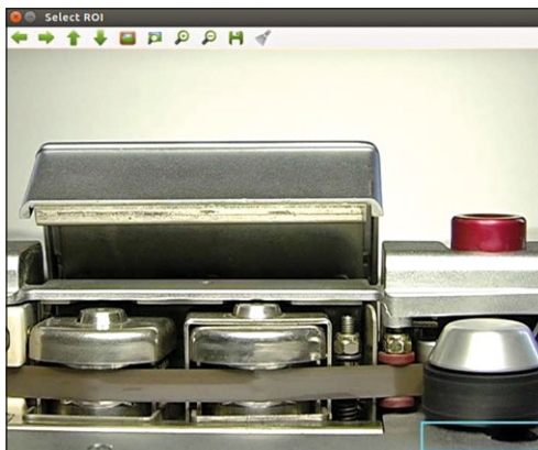
Fig. 3 – Area under the pinch-roller.
