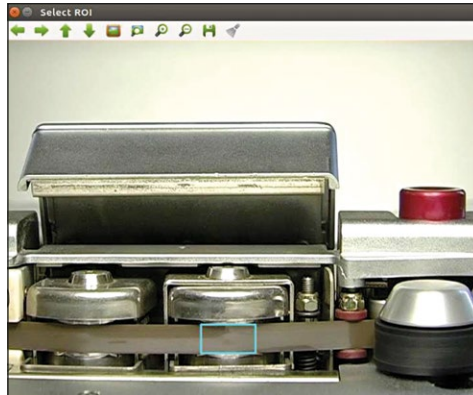
Fig. 2 – Area of the tape recorder reading head.
