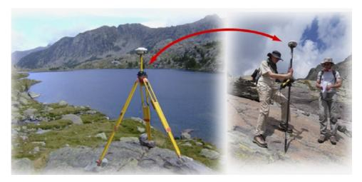
Fig. 1 - Base station receiver at the Lac Long Supérieur, mobile receiver in the valley.
