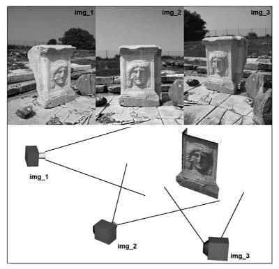
Fig. 3 – Example of the three photographs of the object and virtual representation of the original position of the camera for each photo.
