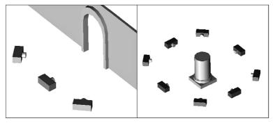
Fig. 2 - Design for monoscopic photogrammetry: 2D object (left) and 3D objects (right).
