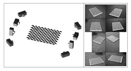
Fig. 1 – Design showing position and orientation of cameras during the photography of the calibration panel, and example of images.
